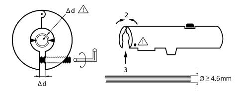
Insert cable, close tool and cut along the cable.
